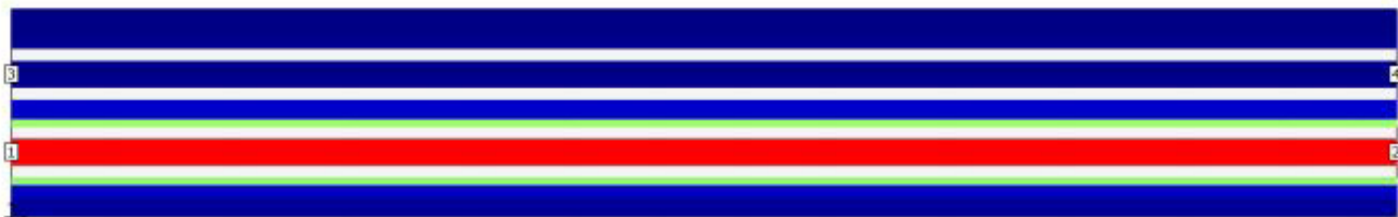
Figure 6a: It is interesting to look at the resulting current densities of the model in Figure 4 when excited. In this plot at 100 MHz there are no resonances present. As can be seen, all the high current is in the aggressor trace and along the edges of the copper pour as would be expected. Red is high-current density while blue is the lower-current density.
