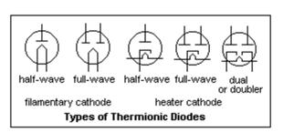
figure. Signal diodes are also often added to a triode or pentode, sharing the same cathode and with one or two plates. Current flows only from plate to cathode, and this unidirectional conduction is the purpose of a diode. Diodes cannot amplify.
