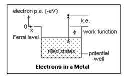
up to some energy called the Fermi energy at 0 K. At ordinary temperatures, there is little difference, since the thermal energy is small compared to the kinetic energy of the electrons near the Fermi level.
