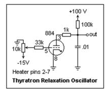
the 884 cannot supply enough current for the usual applications. Larger mercury-vapor thyratrons were manufactured for this service that could handle several amperes.
