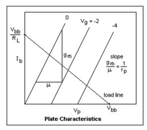
them shows how much the plate current changes for a change in grid voltage. The ratio is a conductance, called the transconductance, denoted by g<sub>m</sub>, measured in siemens (mho). The slope of the curves is the ratio  $g_m/\mu$ , called the *plate conductance*  $g_p$ . With vacuum tubes, the reciprocal  $r_p$ was always used, called the plate resistance. Since actual characteristics are curved, these quantities vary for different currents and voltages.
