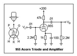
plate voltage is 180V, the maximum cathode current 8 mA. Full ratings apply up to 250 MHz.
