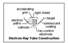
that acts just like the screen grid of a tetrode to create the target current of a few milliamperes. At one side is a *ray-control electrode*, a flat metal strip insulated from the other components. The electrons are accelerated from the space charge region by the accelerating electrode, and then pass into a nearly field-free region where they drift in straight lines to the target, creating light when they strike the phosphor.
