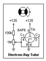
a target voltage of 161 V, 40 V on the control electrode shrunk the dark sector to 45°, and 97 V was enough to close it. One may suppose that a voltage 60% of the target voltage will generally do this.
