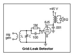
The tuned circuit can be one from a crystal set, with a loopstick and variable capacitor. The signal generator is coupled by about 9 turns slipped over the loopstick, providing an AM signal about 30% modulated with 1 kHz, in the broadcast band. The output was roughly constant, no matter what the plate voltage (45 to 105 V), input amplitude, value of grid resistor (from 1M to 3M) or grid capacitor (100 pF to 220 pF). The grid bias with no signal was about -0.5 V with a 1M grid resistor.
