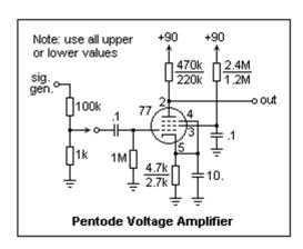
ended, since the 6SJ7 does not have a grid cap. Two sets of values for the components are shown for this amplifier. The upper values give a gain of -164, a plate current of 135  $\mu$ A, a plate voltage of 29V, a screen voltage of 17V, and a grid bias of -0.8V. The lower values give a gain of -117, a plate current of 262  $\mu$ A, a screen voltage of 20V, and a grid bias of -0.9V. It is necessary to have a low plate current
