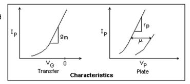
These values are not constant, of course. Verify that  $\mu = g_m r_p$ . Find the cutoff bias for some value of plate voltage. Since this point is not definite, it is usually defined as the voltage at which the plate current drops to some small value, say 10  $\mu$ A.
