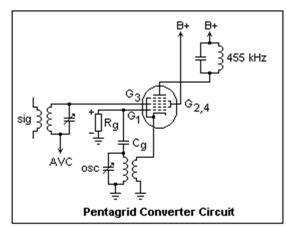
which was the control grid G4, to the plate. G2 was found unnecessary, and was moved to become a suppressor grid, internally connected to the cathode as in a pentode. G1 remained the oscillator grid, but the oscillator plate was represented by the ensemble of G2, G4 and the plate. G2 and G4 are connected internally and screen G3 very tightly.
