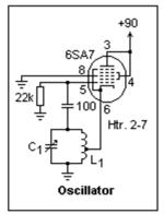
An oscillator using a 6SA7 pentagrid converter is shown at the left. A 6BE6 can be used instead, if you wish. The circuit will not oscillate with an unbypassed resistor in the plate lead, but you can measure the DC plate current with a DMM instead.  $L_1$  is an "oscillator coil" as shown at the right, where terminals 1 and 3 are the ends of the coil, and terminal 2 is a tap,
