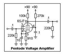
A pentode voltage amplifier using a 6SJ7 is shown at the left. The AC gain of this amplifier is close to  $g_m$  = 1.6 mS times 68.8k, or -110. It won't be quite this high with a 90V B+, but will still give a lot more gain than the triode amplifier. My 6SJ7 gave a gain of -60 at  $V_{bb}$  = 90 V, and  $V_p$  was 27.2 V, showing that the plate current, 0.63 mA, should be reduced a little to raise the plate to about 45 V. The 6SJ7 tested was very close to specifications, despite its age.
