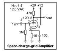
current is 74 mA. These are rather large currents, but the low voltages mean that only modest power is involved. Note that the input impedance is high, set by the 1M grid resistor, and the output resistance is low.
