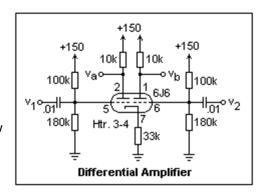
found  $G_D$  = 6.5 (at one plate), and  $G_{CM}$  = 0.15, for a CMRR of 43 or 33 dB. The cathode voltage was 102 V, the total cathode current 3.2 mA. The circuit is probably not optimum, but demonstrates the circuit well, which is also called a "long-tailed pair." With a higher plate voltage, the differential gain could be brought closer to 25.
