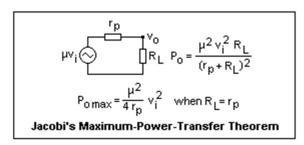
things equal. This is an application of Jacobi's maximum-power-transfer theorem. The power is then given by the square of the input voltage times a factor called the *power sensitivity*,  $\mu^2/4r_p$ .
