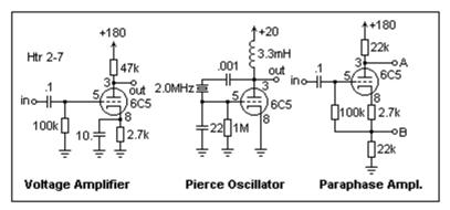
47k||11k and the transconductance of 1.8 mS. The plate current was 1.67 mA. As usual, small plate currents are used in voltage amplifiers so that the plate resistor can be as large as possible.
