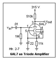
can be used for amplification. This diagram also gives the pin connections for the tube.
