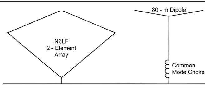
Fig 12—Combination of the N6LF array and an 80-meter dipole for modeling.
