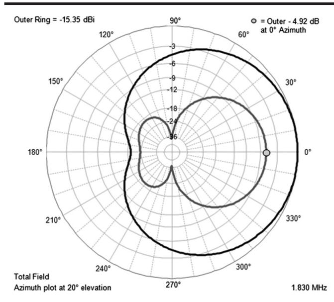
Figure 8 — 1.83 MHz azimuth plot at 20°.
