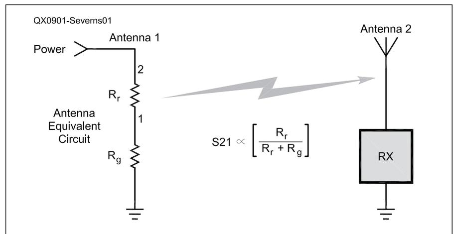
Figure 1—This drawing illustrates the traditional measurement scheme.
