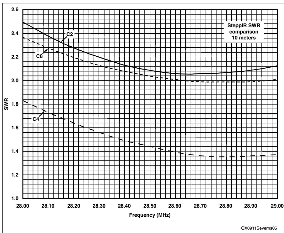
Figure 5 — Feed point SWR comparison on 10 m.
