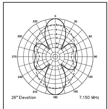
Fig 1—Azimuth pattern of classic double extended Zepp (solid line) at 7.15 MHz, compared with standard dipole (dashed line), both 80 feet high over average ground. Patterns are shown at  $26^\circ$  elevation, where the gain is maximum. The wire runs along the  $270^\circ$  to  $90^\circ$  axis on the graph. Note significant sidelobes for DEZepp.
