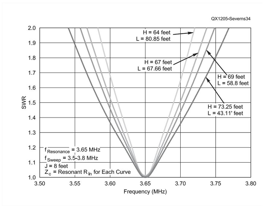
Figure 34 — SWR with  $Z_0$  equal to  $R_{\text{in}}$  at resonance for the particular combination of H and L.
