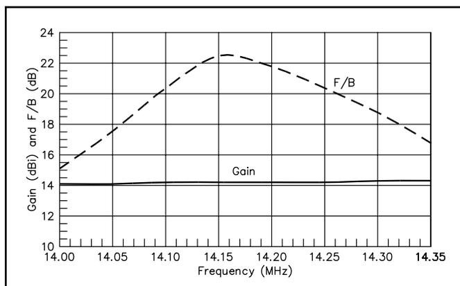
Fig 5—Gain and F/B characteristics on 20 meters.
