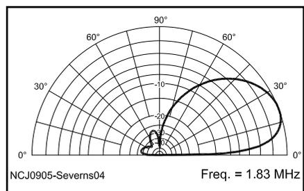
**Figure 5 — N6LF array elevation pattern at 0° azimuth**
