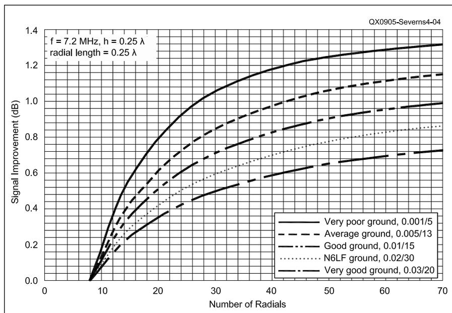
Figure 4 — Calculated signal improvement as we vary the number of radials over different soils with a  $\frac{1}{4} \lambda$  vertical with  $\frac{1}{4} \lambda$  radials at 7.2 MHz. Note: 0 dB is for the 8 radial case.
