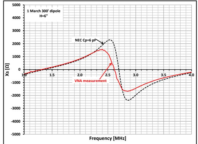
Figure 13 — Reactance measurement at antenna height of 6 inches.
