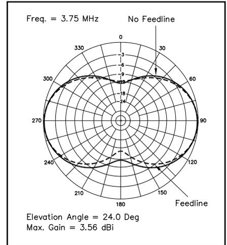
**Fig 14—**Effect of feed line on azimuth radiation pattern for current-fed half-square antenna. The feed line introduces only small distortions in symmetrical radiation pattern. The coaxial feed line was modeled as being brought out straight for 30 feet from the corner, then brought down close to ground level and led away for 50 feet more, where it was grounded.
