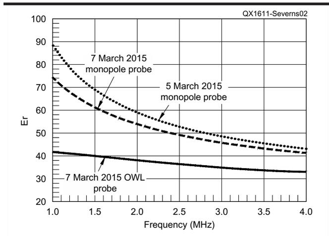
Figure 2 — Soil relative permittivity  $E_r$  at N6LF.
