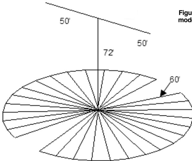
Figure 3 — EZNEC model of the 1BCG antenna.
