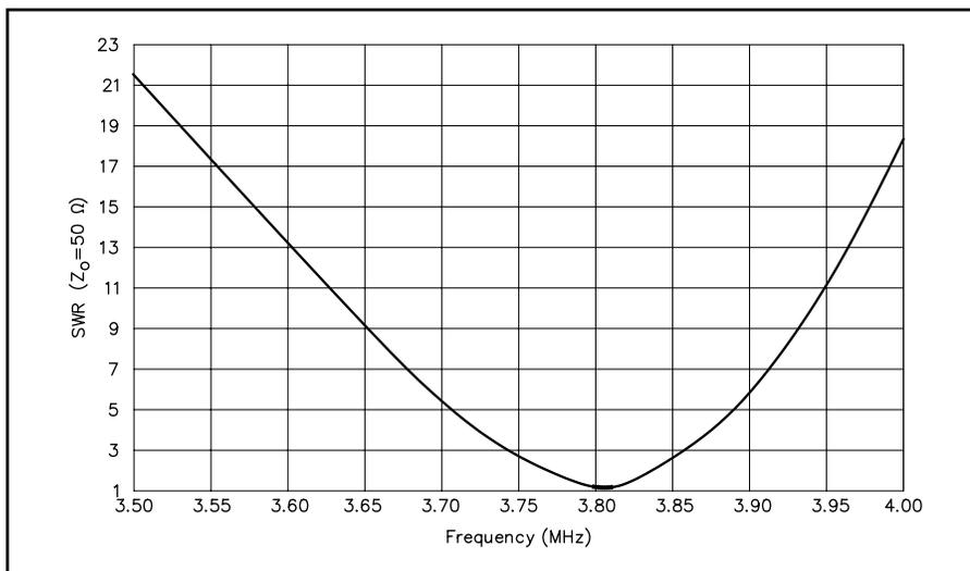
**Fig 15—**SWR versus frequency for voltage-fed half-square antenna, using matching network shown in Fig 10B, with  $L = 15 \mu\text{H}$ ,  $C_1 = 125 \text{ pF}$  and  $C_2 = 855 \text{ pF}$ . The SWR bandwidth is less than 100 kHz at the 2:1 SWR points.
