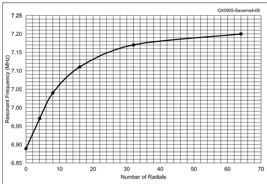
Figure 6 — Resonant frequency of a vertical antenna resonated at 7.2 MHz with sixty four 33 foot radials, as a function of the number of radials.
