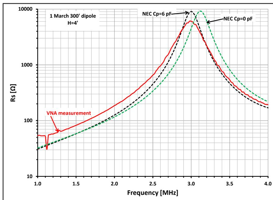
Figure 4 — Modeling with and without  $C_p$ .
