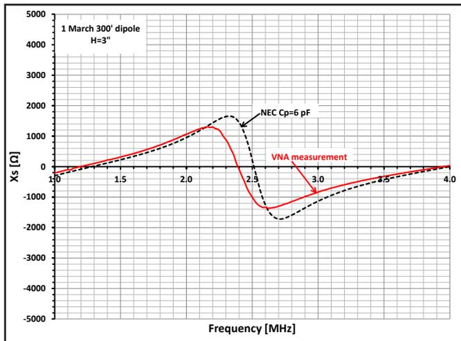
Figure 15 — Reactance measurement at antenna height of 3 inches.
