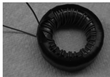
Figure 19 — Secondary winding on the impedance transformer.
