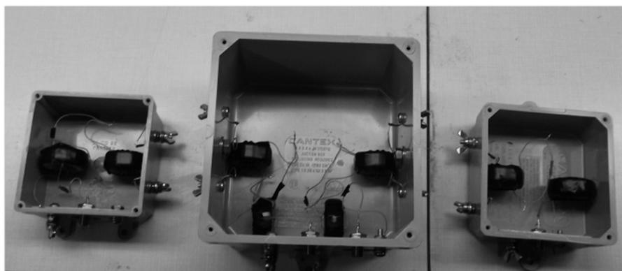
Figure 22 — Feed point boxes with transformer-chokes installed.
