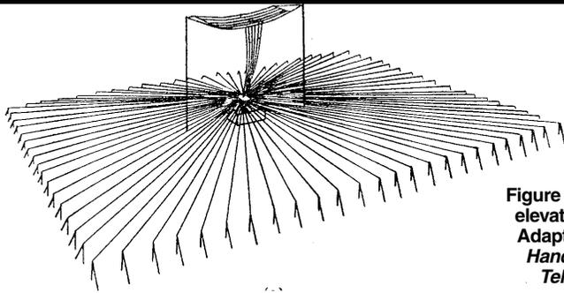
Figure 2 — A very large LF elevated ground system. Adapted from *Admiralty Handbook of Wireless Telegraphy*, 1932.<sup>34</sup>
