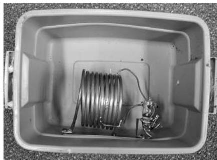
Figure 3 — Relay and base inductor example
