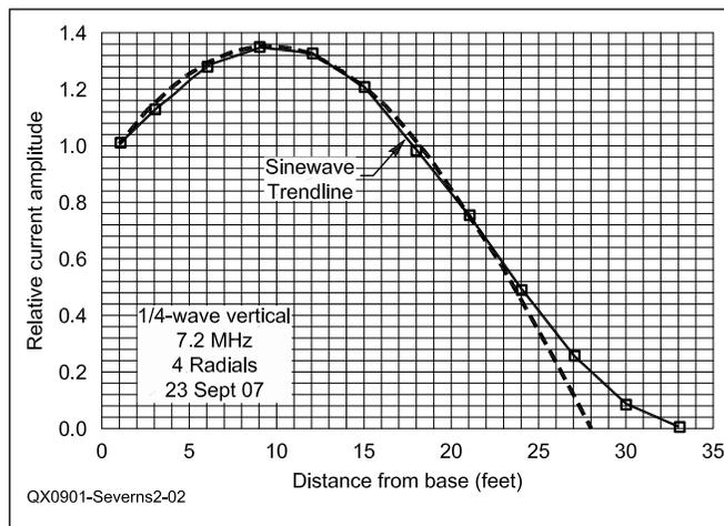
**Figure 2** — This graph shows the relative current amplitude along a radial.
