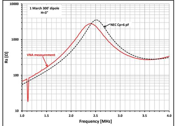
Figure 14 — Resistance measurement at antenna height of 3 inches.
