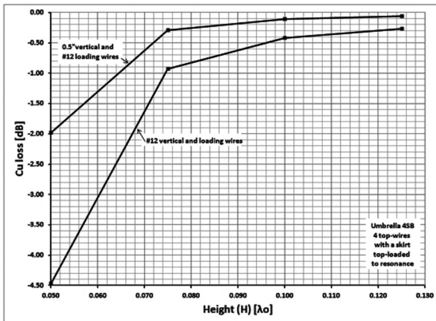
Figure 22 — Examples of conductor loss in short antennas.
