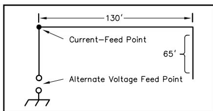
**Fig 2—Typical 80-meter half-square, with  $\lambda/4$ -high vertical legs and a  $\lambda/2$ -long horizontal leg. The antenna may be fed at the bottom or at a corner. When fed at a corner, the feed point is a low-impedance, current-feed. When fed at the bottom of one of the wires against a small ground counterpoise, the feed point is a high-impedance, voltage-feed.**
