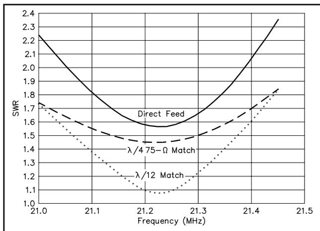
**Fig 9**—Solid line shows 15-meter 50-Ω SWR with direct feed. Dashed line shows 15-meter 50-Ω SWR with quarter-wave 75-Ω matching section. Dotted line shows 15-meter 50-Ω SWR with a series transformer match.
