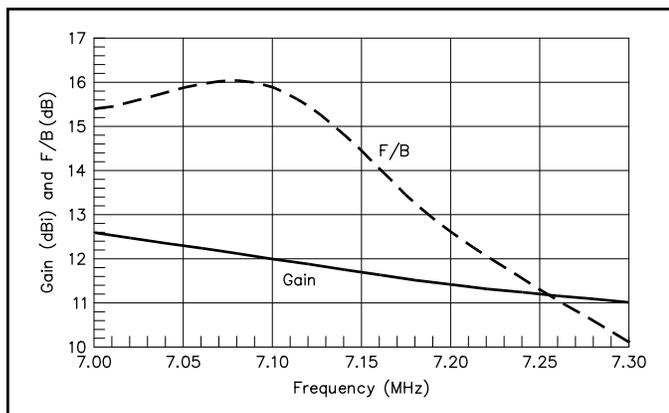
Fig 4—Gain and F/B characteristics on 40 meters.
