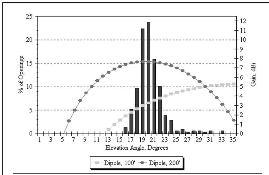
Fig 1—80-meter graph of the percentage of all openings from New England to Europe versus elevation angles, together with overlay of elevation patterns over flat ground for dipoles at two different heights. The 200-foot high dipole clearly covers the necessary elevation angles better than does the 100-foot high dipole. (From *The ARRL Antenna Book*, 17th edition, Fig 30.)
