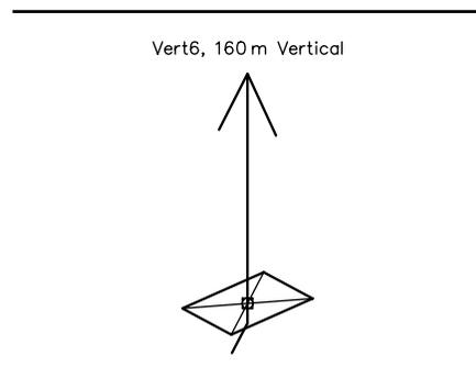
Fig 5—Antenna configuration.
