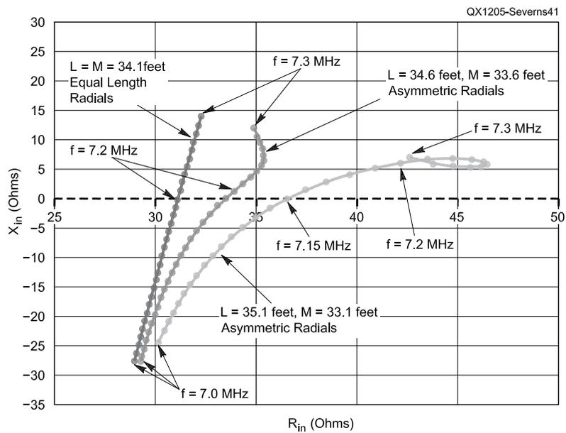
**Figure 41 — A comparison of the input impedances ( $Z_{in} = R_{in} + jX_{in}$ ) from 7.0 to 7.3 MHz at the feed point of the vertical, for symmetric and asymmetric radial lengths. The frequency is stepped in 10 kHz increments.**
