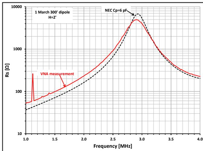
Figure 8 — Resistance measurement at antenna height of 24 inches.
