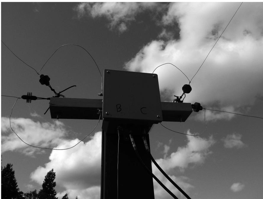
Figure 23 — Transformer box at the center of the array.
