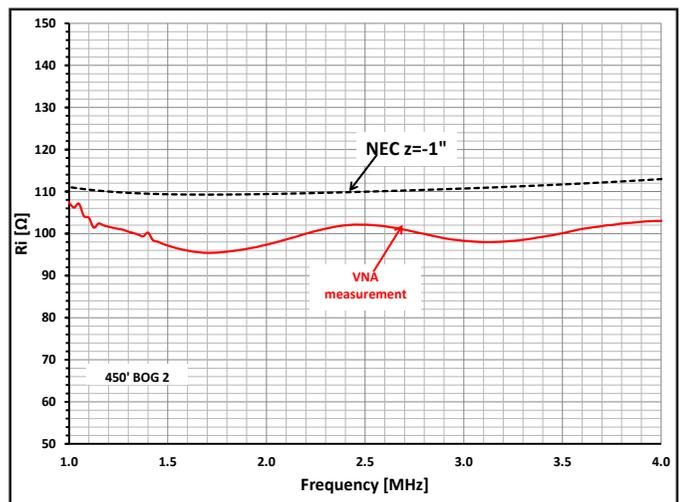
Figure 36 — Measured and computed BOG resistance.
