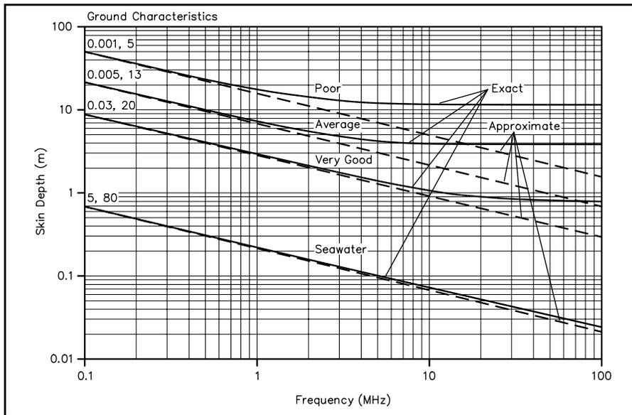
Figure 12—Skin depth in soil of various characteristics as a function of frequency.
