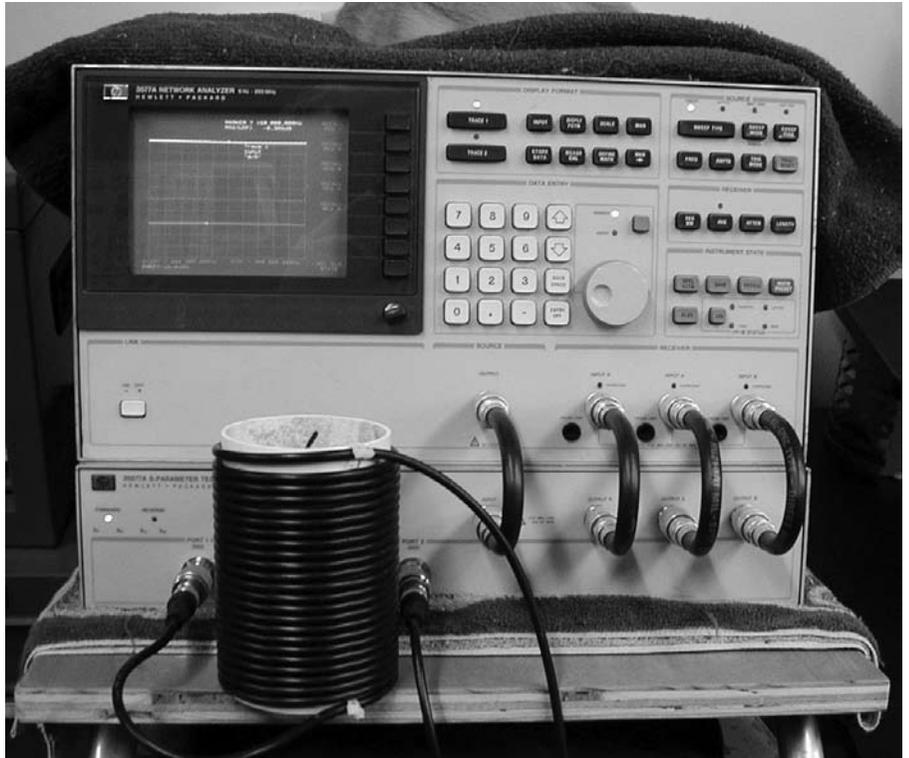
Figure 9 — HP3577A with an HP35677A S-parameter test box.
