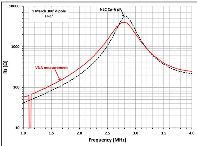
Figure 10 — Resistance measurement at antenna height of 12 inches.
