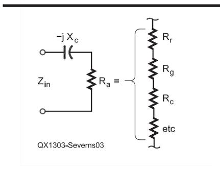
Figure 3 — Equivalent circuit for  $Z_{in}$ .
