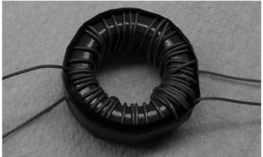
Figure 20 — Primary winding added to the impedance transformer.
