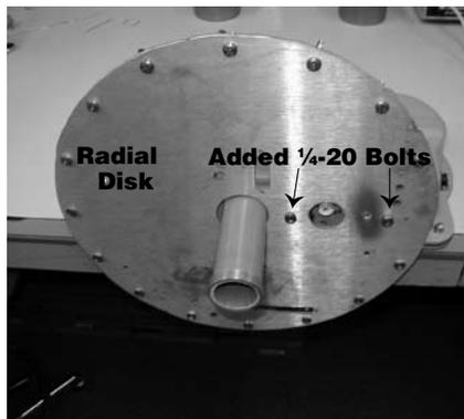
Figure 2A — SteppIR with radial disk attached.
