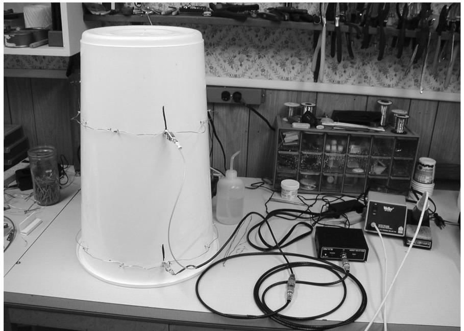
Figure 2 — Calibration test fixture shows the AIM4170 as the VNA, but the same fixture was used to calibrate the N2PK vector network analyzer that was used for the actual measurements.
