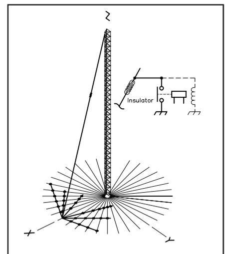
Figure 6—A simple 2-element slant-wire parasitic array.
