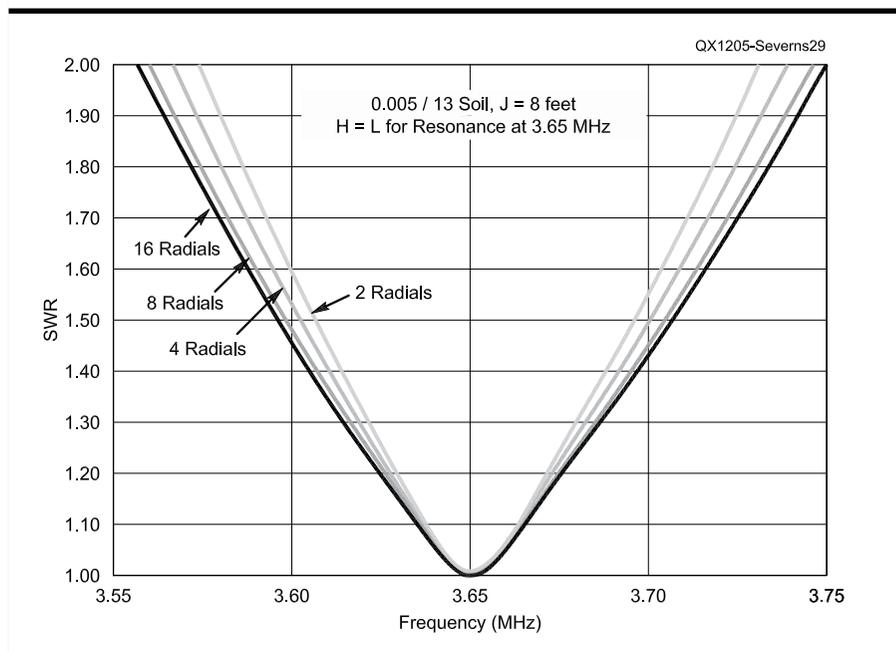
Figure 29 — Feed point SWR as a function of N.
