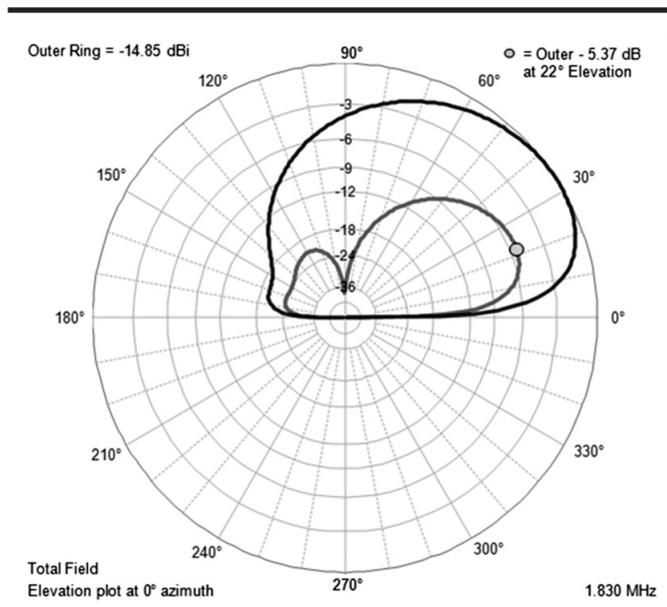
Figure 9 — 1.83 MHz elevation plot.
