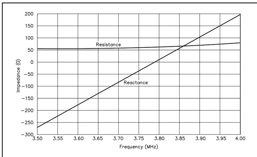
**Fig 12—Graph of feed point series resistance and reactance versus frequency for a half-square with current-feed at one corner. Note that the resistive component changes slowly with frequency. This particular antenna is resonant at just under 3.8 MHz.**
