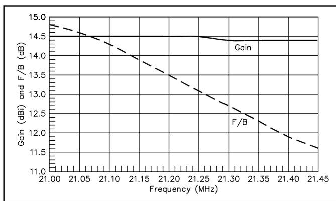
Fig 6—Gain and F/B characteristics on 15 meters.
