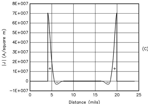
**Fig 2—Current density ( $J$ ) in a solid copper #26 AWG wire (cross section A) at 1 (B) and 16 (C) MHz.**
