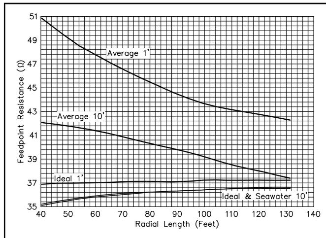
**Fig 4—Feed-point resistance as a function of radial length and radial height above ground. Here, the loss resistance of the loading inductor is removed. The effect of ground loss over soil is large compared to that over salt water.**
