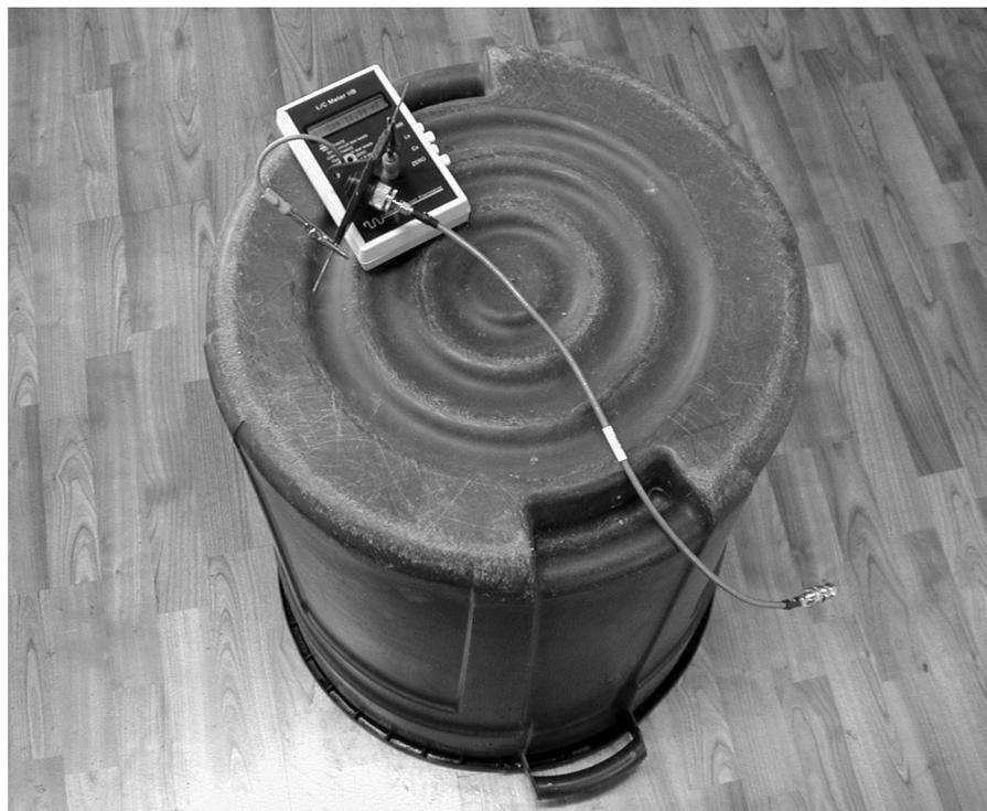
Figure 3 — Shunt capacitance measurement of the center fitting.
