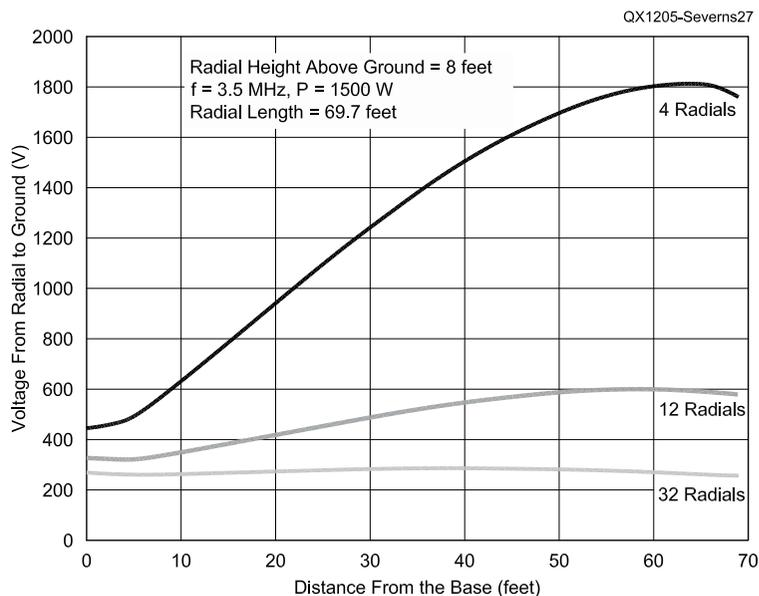
**Figure 27 — Examples of the voltage from a radial wire to ground with different numbers of radials. The input power to the vertical is 1500 W, the operating frequency is 3.5 MHz and the radial system is elevated 8 feet above ground.**
