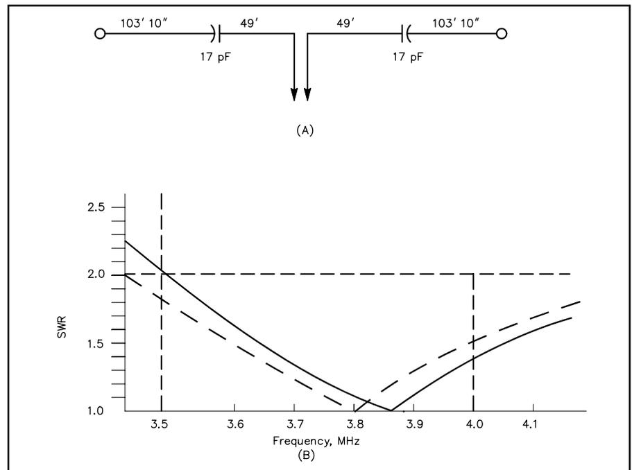
Fig 8—75/80-meter N6LF DEZepp, designed using *NEC Wires*. At A, a schematic is shown for antenna. At B, SWR curve is shown across 75/80-meter band. Solid line shows measured curve for W7ISV antenna, which was pruned to place SWR minimum higher in the band. The dashed curve shows the computed response when SWR minimum is set to 3.8 MHz.
