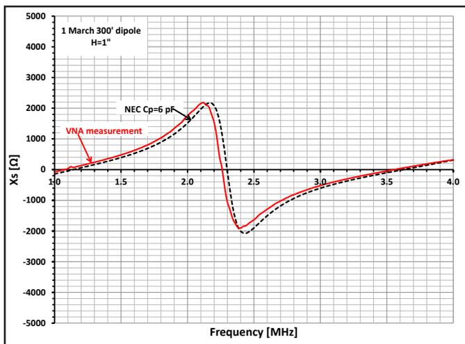
Figure 17 — Reactance measurement at antenna height of 1 inches.
