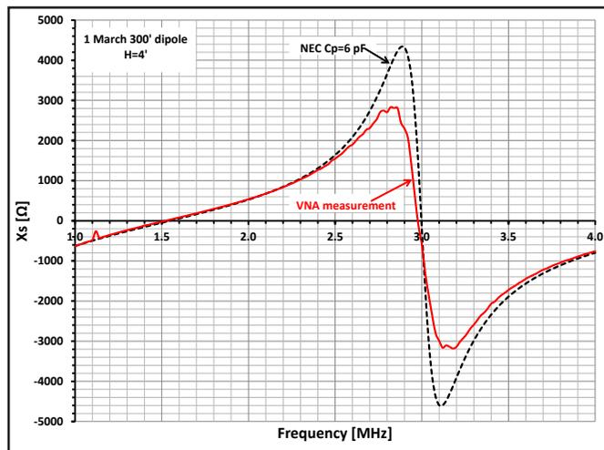
Figure 7 — Reactance measurement at antenna height of 48 inches.
