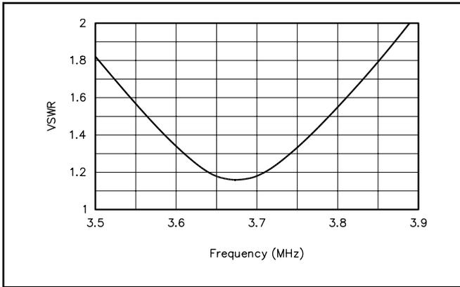
Figure 5—The SWR plot for the N6LF Bruce array.
