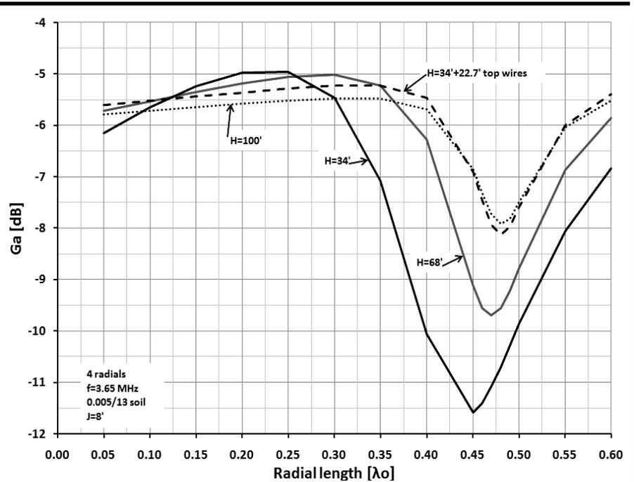
Figure 18 — Effect on  $G_a$  of short verticals.  $H = 100$  feet, 68 feet, 34 feet and 34 feet with top-loading.
