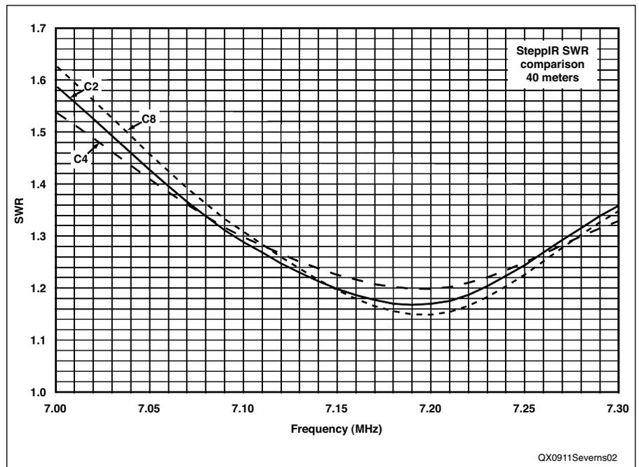
**Figure 2 — Feed point SWR comparison on 40 m.**
