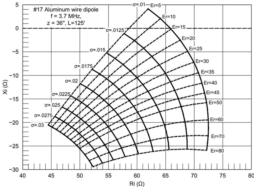
Figure 6 —  $X_i$  versus  $R_i$  for  $0.01 < \sigma < 0.03$  and  $5 < E_r < 80$ .
