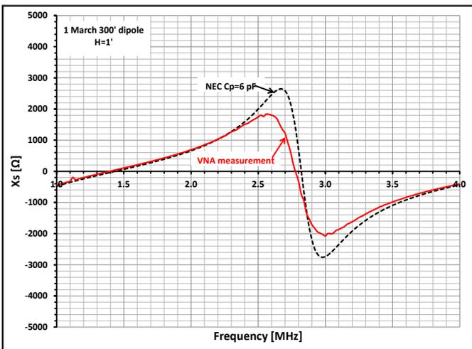
Figure 11 — Reactance measurement at antenna height of 12 inches.
