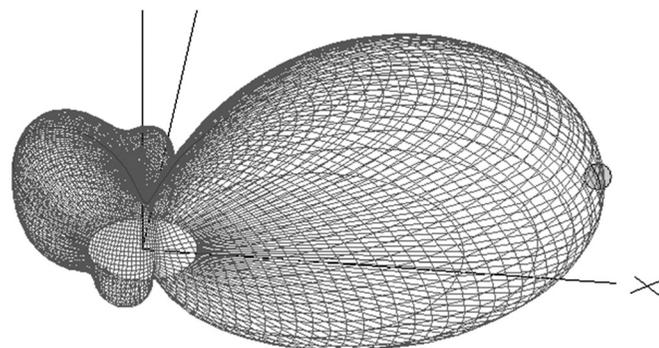
Figure 18 — 3-D pattern for four loops.
