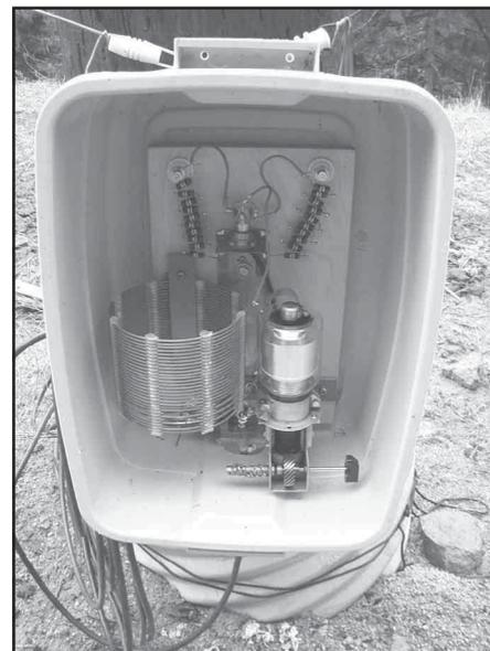
Fig 11—Photograph of the tuner.
