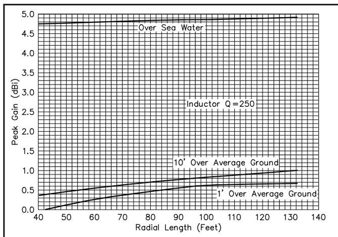
**Fig 1**—Peak gain for  $\lambda/4$ -high vertical with four, coil-loaded short radials on 160 meters. The loading coil is assumed to have an unloaded Q of 250. Over seawater, the peak gain doesn't change much, even for quite short radials, while the gain is close to 5 dB less over ground with average conductivity and dielectric constant.
