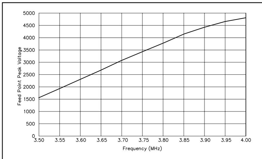
**Fig 11—Graph of peak RF voltage at feed point of voltage-fed half-square antenna with 1500 W power.**
