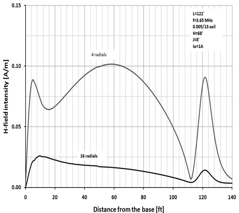
Figure 25 — E and H field intensities close to the ground surface directly below the radials. N = 4 and 16.
