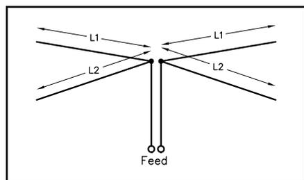
Fig 1—Broadbanding an 80-meter dipole using a fan-shaped pair of unequal-length radiators.
