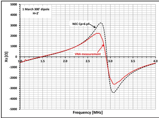
Figure 9 — Reactance measurement at antenna height of 24 inches.
