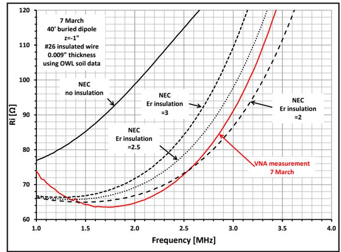
Figure 27 — Effect of wire insulation relative dielectric constant.
