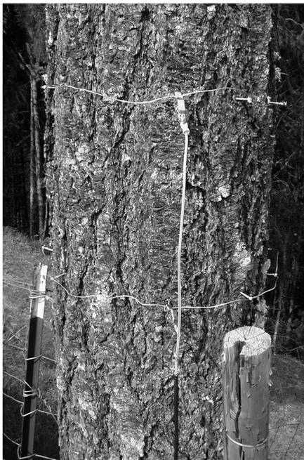
Figure 1 — Impedance measurement on a Douglas fir tree.
