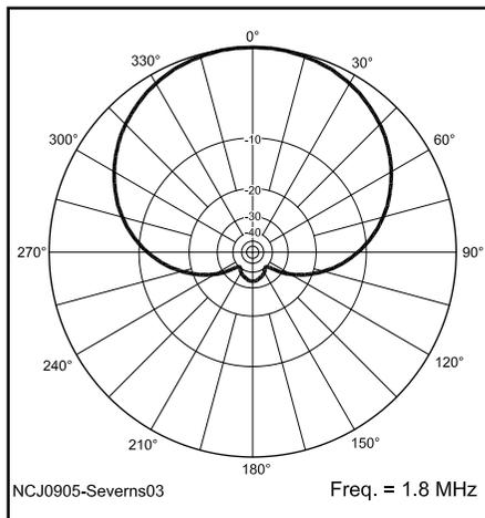
**Figure 4 — N6LF array azimuth pattern at 20° elevation**
