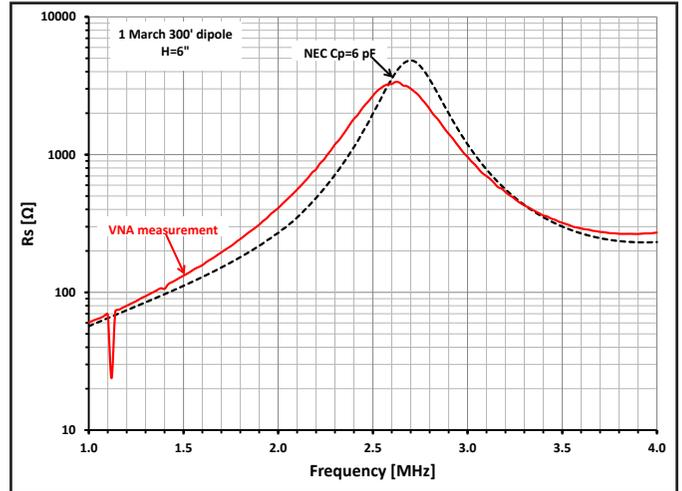
Figure 12 — Resistance measurement at antenna height of 6 inches.
