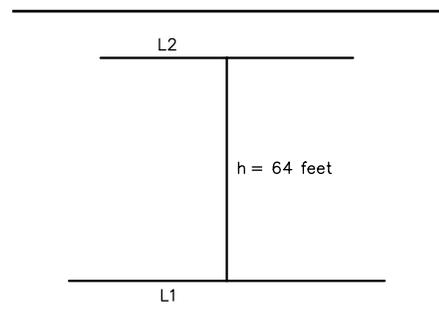
Fig 3—Asymmetric two-radial dipole.  $F_R = 3.790$  MHz.
