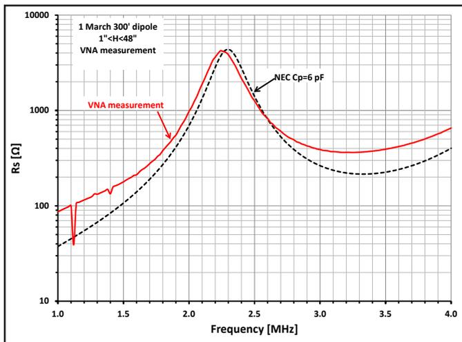
Figure 16 — Resistance measurement at antenna height of 1 inches.
