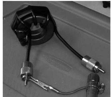
Figure 3A — Common mode choke for the feed line.
