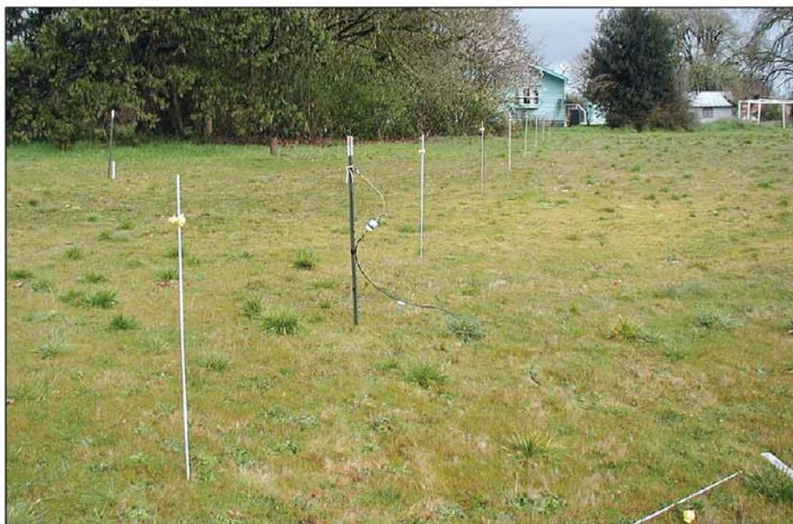
perimentally validate *NEC-4.2* modeling before I could confidently move on to my BOG problem. I performed a series of experiments with actual antennas having wires parallel to the soil at low heights,
