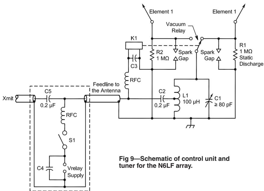
Fig 9—Schematic of control unit and tuner for the N6LF array.
