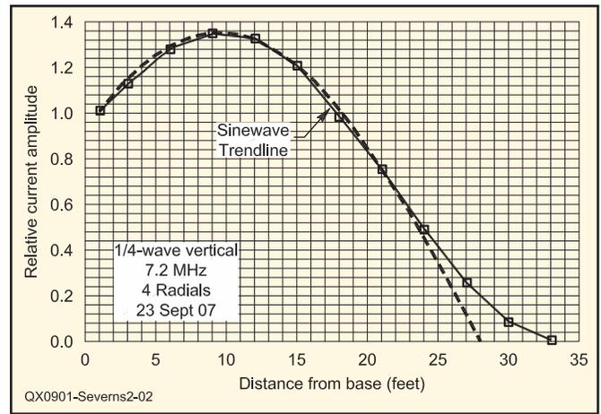
**Figure 3 — Measured current distribution on a radial.**
