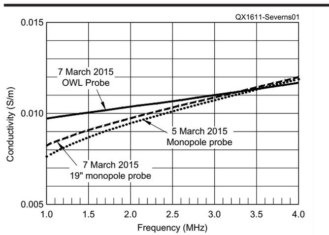
Figure 1 — Soil conductivity  $\sigma$  at N6LF.
