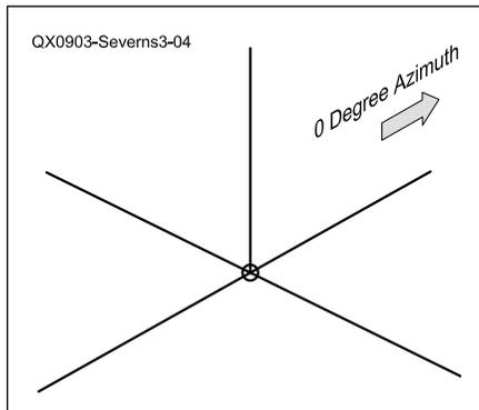
Figure 4 — Four elevated radials, 48 inches above 0.015/30 soil.
