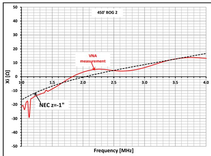
Figure 37 — Measured and computed BOG reactance.
