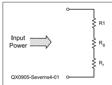
**Figure 1 — An antenna input equivalent circuit.  $R_l$  represents the ohmic loss due to conductors, loading inductor series resistance, and so on.  $R_g$  represents the power dissipated in the soil by the near-field of the antenna.  $R_r$  is the radiation resistance, which accounts for the radiated power.**
