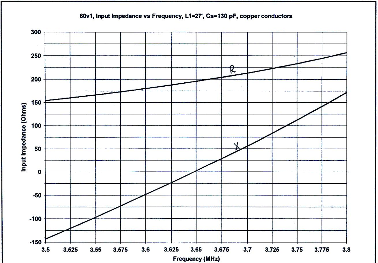
Figure 10. Feedpoint resistance and reactance from 3.5 to 3.8 MHz.
