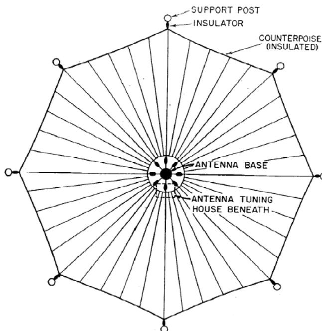
Figure 1 — A typical counterpoise ground system. Figure adapted from from Laport.<sup>14</sup>
