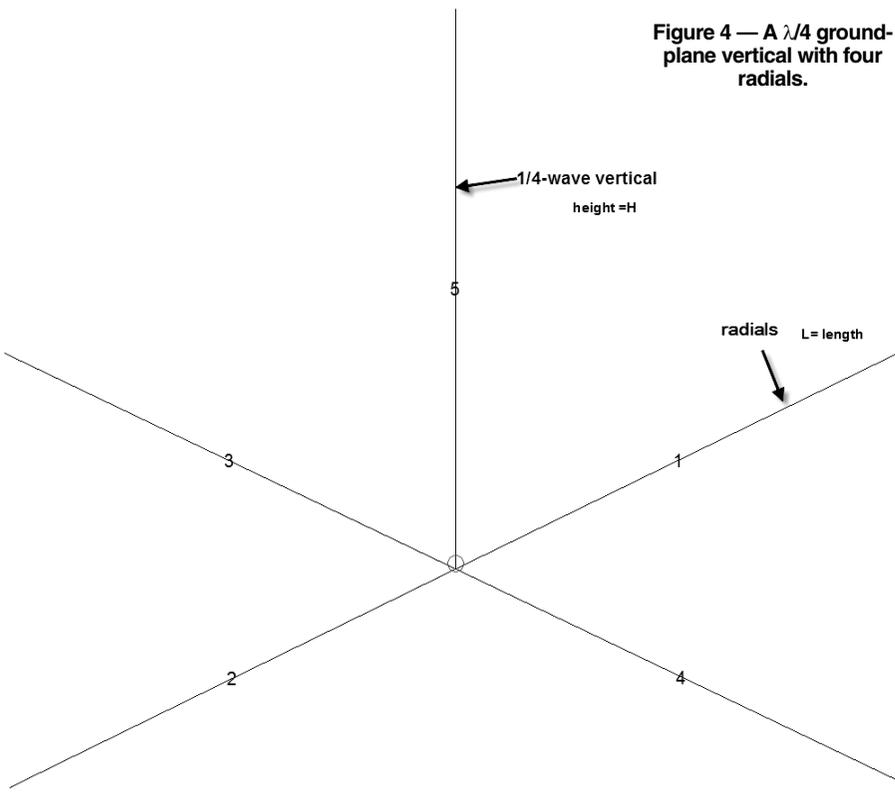
Figure 4 — A  $\lambda/4$  ground-plane vertical with four radials.
