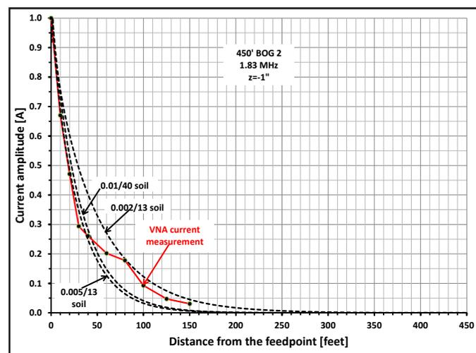
Figure 38 — Measured and computed BOG current amplitude.
