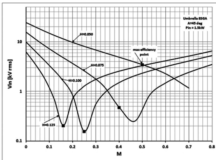
Figure 23 — Feed point voltage as a function of M with H = 0.050, 0.075, 0.100 and 0.125.
