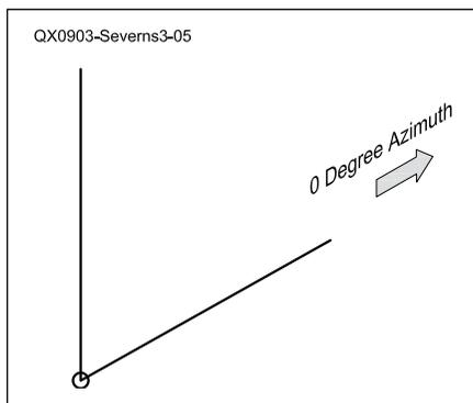
Figure 5 — One elevated radial, 48 inches above 0.015/30 soil.
