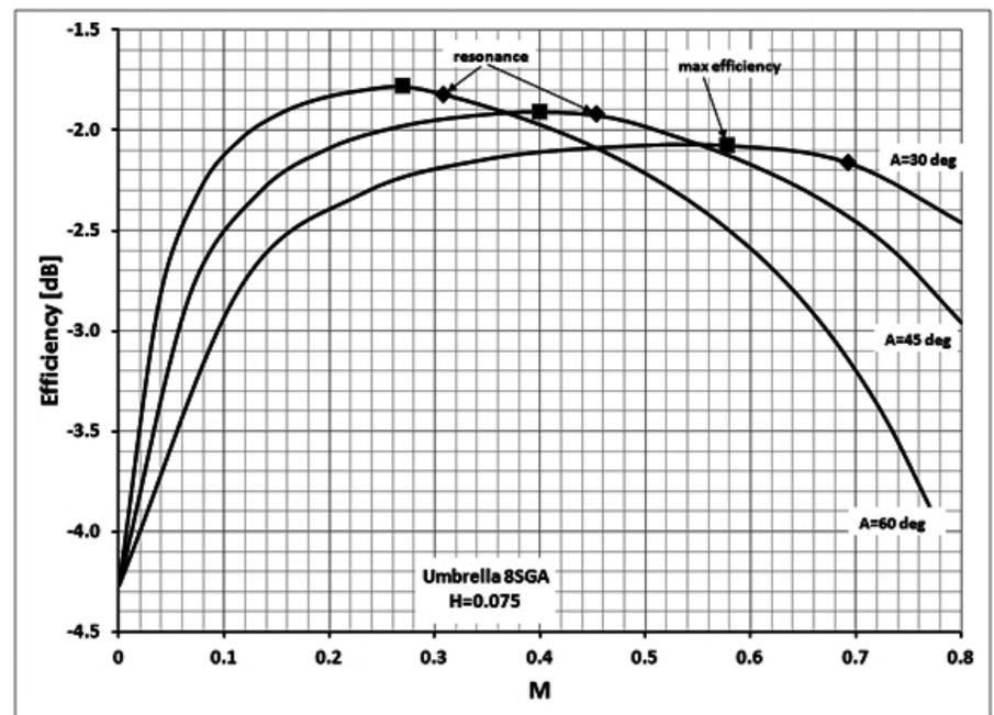
Figure 19 — Efficiency in dB as a function of M with A as the parameter and  $H = 0.075$ .
