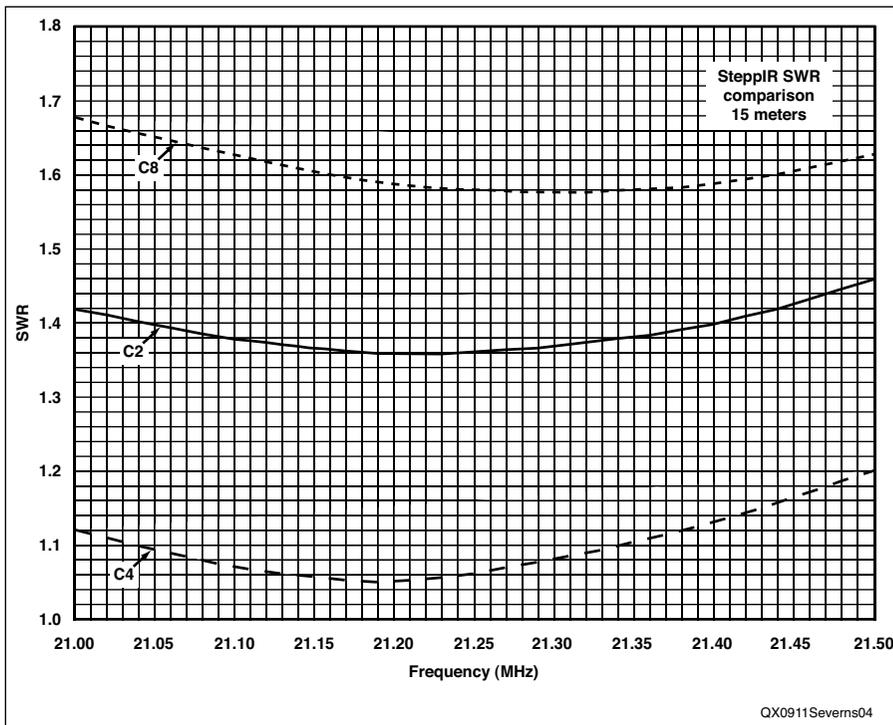
**Figure 4 — Feed point SWR comparison on 15 m.**
