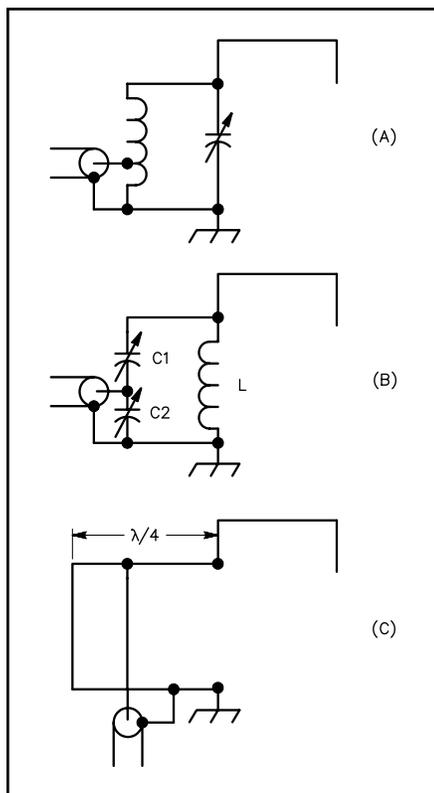
**Fig 10—Typical matching networks used for voltage-feeding a half-square antenna.**
