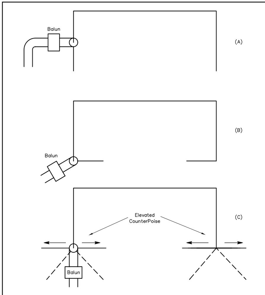
**Fig 16—Possible methods for current-feeding of half-square antenna at points other than the upper corners. At A, a balun is used to decouple the feed line from the feed point at the center of one of the vertical legs of the antenna. At B, the ends of the vertical legs are both bent back horizontally to provide a feed point. At C, an elevated counterpoise is used to provide a feed point at the bottom of a vertical leg.**
