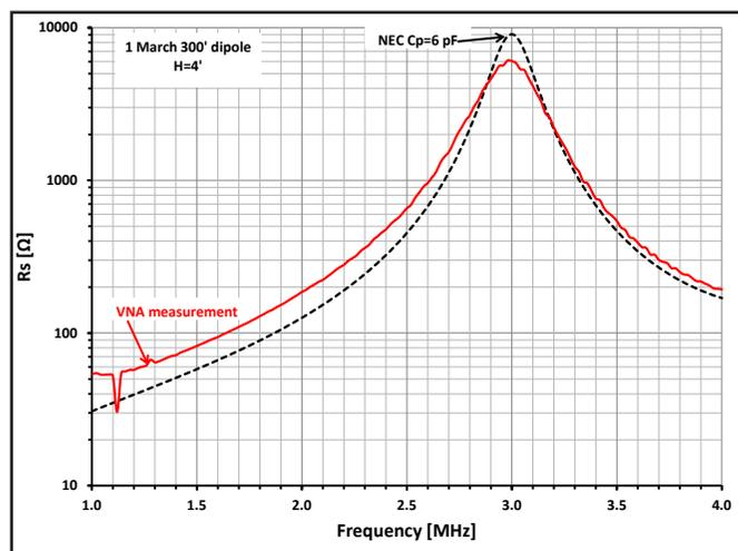
Figure 6 — Resistance measurement at antenna height of 48 inches.
