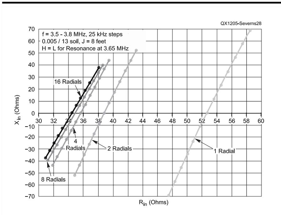
Figure 28 —  $X_{in}$  versus  $R_{in}$  ( $Z_{in} = R_{in} + j X_{in}$ ) where frequency varies from 3.5 MHz (lower left ends of the curves) to 3.8 MHz (upper right ends of the curves) for different values of N. Frequency is stepped in 25 kHz intervals.
