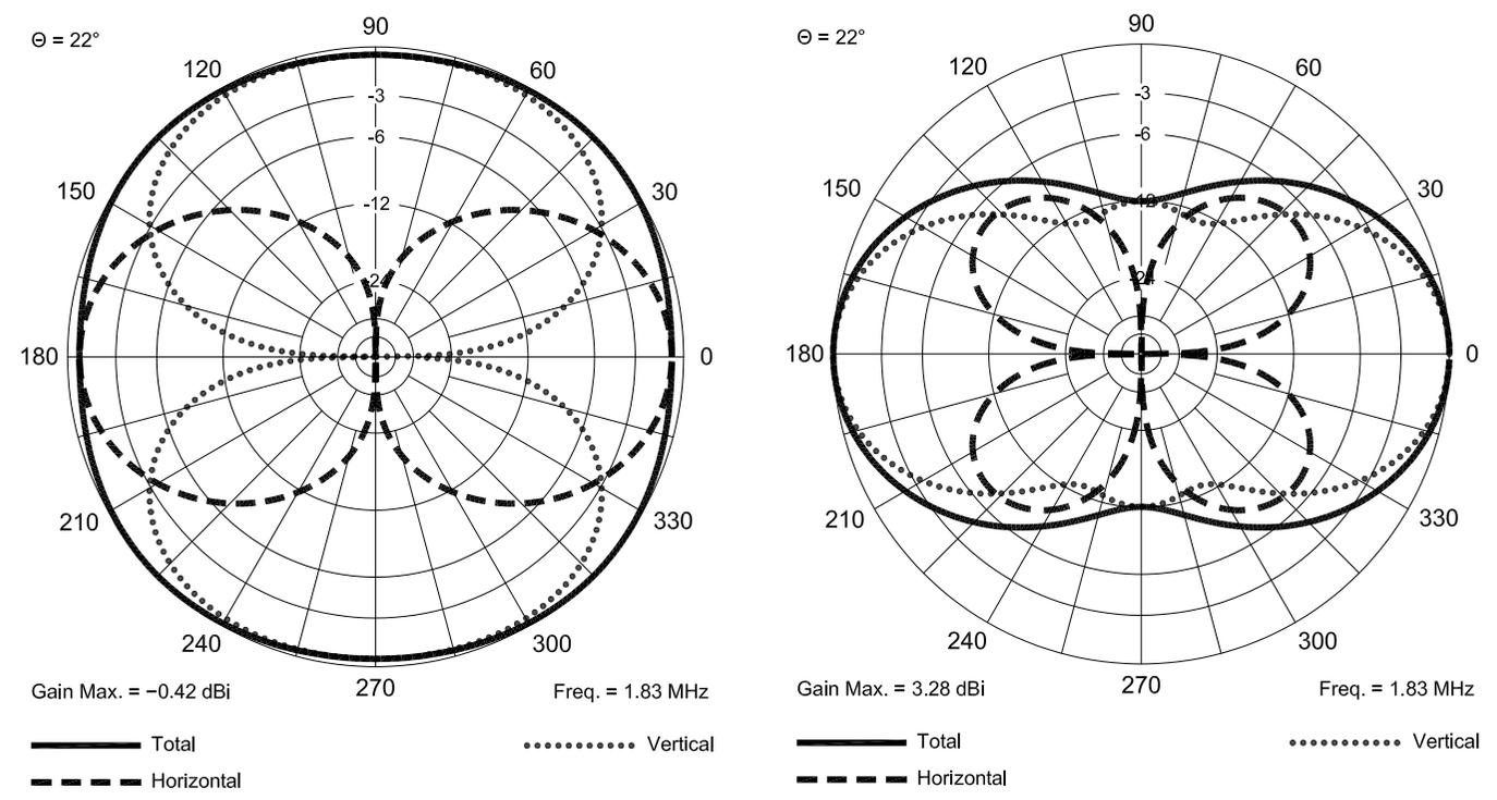
Fig 6—Vertical, horizontal and total pattern at 22° elevation for two half-wave slopers. At A, driven in-phase and at B, 180° out of phase, with the upper ends at 150 feet.
