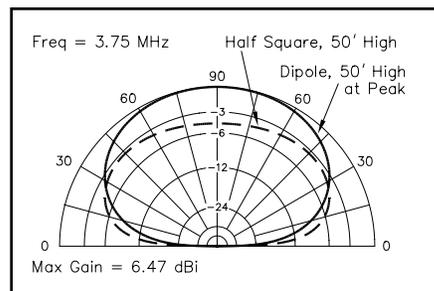
**Fig 8**—Elevation pattern for the asymmetrical half-square shown in Fig 7, compared with pattern for a 50-foot high dipole. This is over average ground, with a conductivity of 5 mS/m and a dielectric constant of 13. Note that the zenith-angle null has filled in and the peak gain is lower compared to conventional half-square shown in Fig 5 over the same kind of ground.
