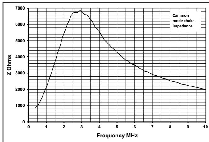
Figure 5 — Measured impedance of the common mode choke.
