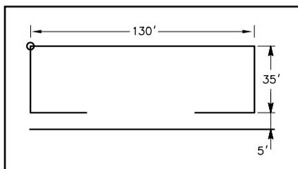
**Fig 3—An 80-meter half-square configured for 40-foot high supports. The ends have been bent inward to resonate the antenna. The performance is compromised surprisingly little.**
