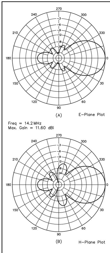
Fig 1—W0H7H 6 element 20-meter quad, free-space radiation patterns. At A, E-plane pattern and at B, H-plane pattern.
