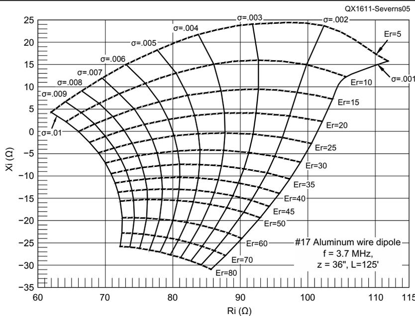
Figure 5 —  $X_i$  versus  $R_i$  for  $0.001 < \sigma < 0.01$  and  $5 < E_r < 80$ .
