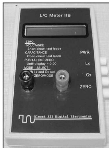
**Figure A1 — I used this Almost All Digital Electronics L/C meter to measure the capacitance of the probes in air. By measuring the total capacitance of the probe and leads, and then measuring the parasitic capacitance, C<sub>p</sub>, of the part of the probe above ground along with the connecting leads, I am able to calculate the capacitance of the probe alone, C<sub>0</sub>.**
