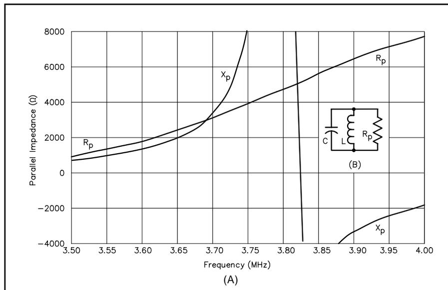
**Fig 9**—At A, graph of feed point shunt resistance and shunt reactance versus frequency for a half-square with voltage-feed at bottom corner. At B, equivalent parallel circuit of this antenna. This particular half-square is resonant at about 3.820 MHz, where its feed point resistance is about 5000 Ω.
