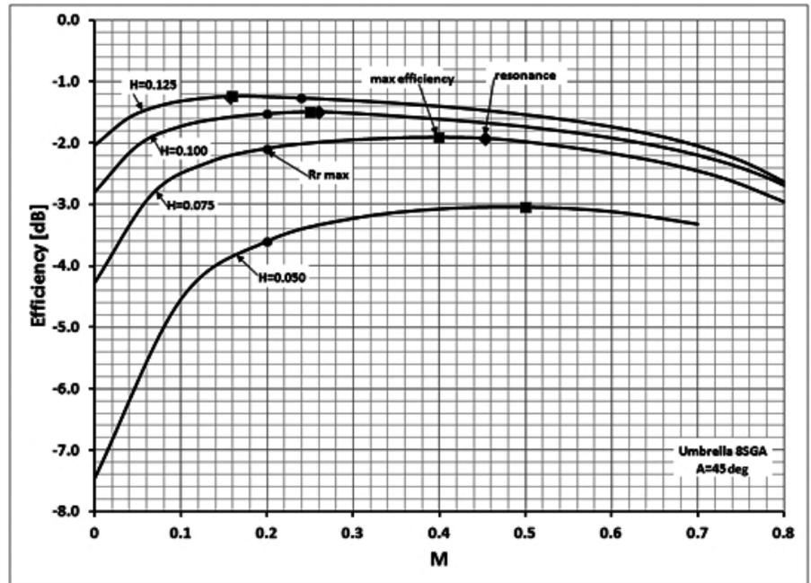
Figure 18 — Efficiency in dB as a function of M with H as the parameter and  $A = 45^\circ$ .
