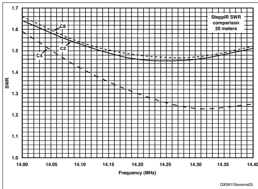
**Figure 3 — Feed point SWR comparison on 20 m.**
