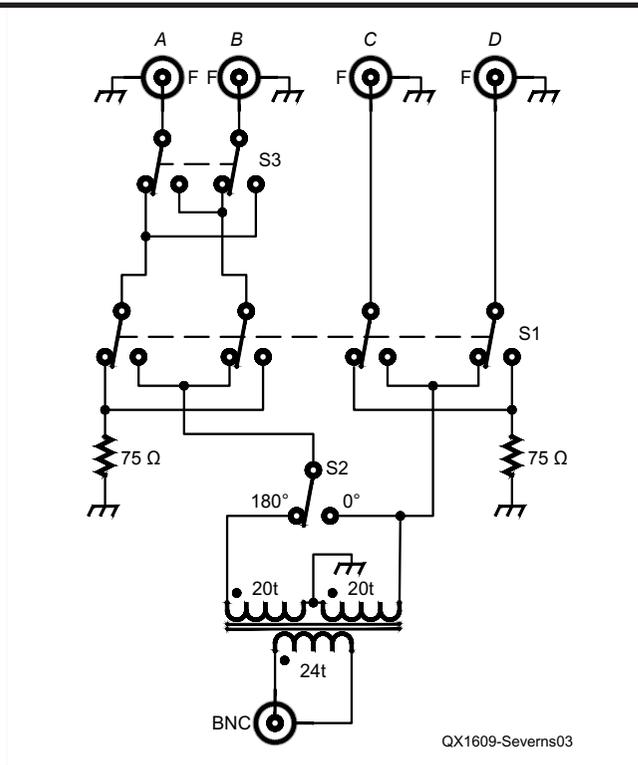
Figure 3 — Control unit schematic. F-connectors are used at *A*, *B*, *C* and *D* in the 75 Ω portion of the system, and a BNC connector is used at the 50 Ω connector to the receiver.
